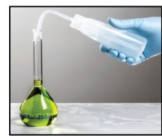
Figure 2 Volumetric flasks are used to make up solutions. They have a graduation mark around their narrow necks. Water is added to the solute until the bottom of its meniscus (the curve at the surface of the solution when viewed from the side) is level with the mark
