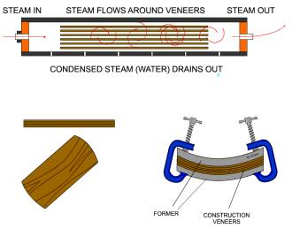
This process enables curved products to be manufactured. Lamination is the process of layering thin pieces of wood on top of each other with an adhesive between each layer.
