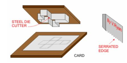
The steel die cutter is made up of specially hardened steel cutters. Each is like a blade, with a serrated edge. Sometimes the blades can be rearranged to form other shapes of net.
