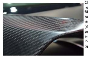
CFRP is an extremely strong and light fibrereinforced plastic which contains carbon fibres. CFRPs can be expensive to produce but are commonly used wherever high strength-to-weight ratio and stiffness (rigidity) are required, such as aerospace, superstructure of ships, automotive, civil engineering, sports equipment, and an increasing number of consumer and technical applications.
