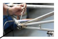
Hard soldering requires higher temperatures (usually flame), it leads to a stronger join.
