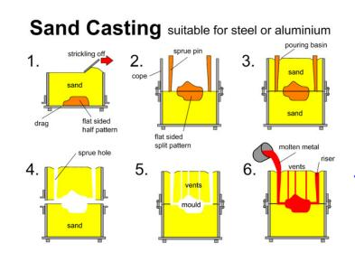
This involves packing a moulding material (traditionally a mixture of sand and clay) around a pattern of the casting. This is usually made of a hardwood and will be larger than the requirements of the finished casting to allow for shrinkage. The mould is then split so that the pattern can be removed.
