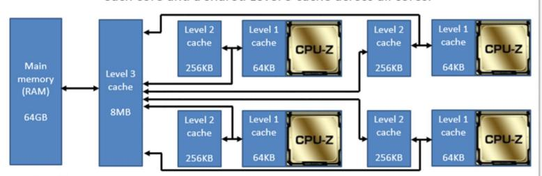
**Level 1 Cache:** Often located directly on the CPU itself, very low capacity, very expensive, typically runs at the same speed as the CPU.
