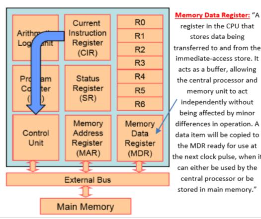
register in the CPU that stores data being transferred to and from the immediate-access store. It acts as a buffer, allowing the central processor and memory unit to act independently without being affected by minor differences in operation. A data item will be copied to the MDR ready for use at the next clock pulse, when it can either be used by the
