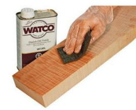
Danish oil, often referred to as an oil finish, is actually a thin oil and varnish mixture. The oil helps bring out wood's beauty, while the varnish resin offers somewhat more protection against chemicals, heat, scratches and stains than either oil or wax. It comes in a variety of
