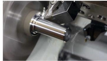
The downside to manual turning is it requires continuous supervision. Automatic turning does not. With Computer Numerical Control, or CNC, you program all the movements, speeds, and tooling changes into a computer. These instructions then get sent to the lathe for completion. CNC allows for consistency and efficiency of high production runs.
