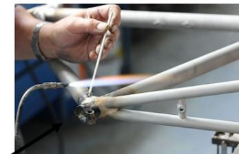
Hard soldering requires higher temperatures (usually flame), it leads to a stronger join.
