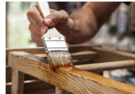
Acrylic Varnish is a clear, high-build wood lacquer, particularly well suited to areas where a high build with exceptional clarity is required, yet a high degree of physical and chemical resistance is not such as wooden bedroom furniture, skirting boards, architraves and other interior trim, fixtures and fittings.
