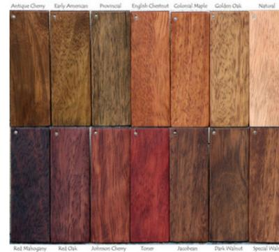
A wood stain penetrates the wood, meaning it colours the wood without obscuring the grain. Woodstains are slightly different to wood paint, in that it brings out the beauty of the wood grain instead of covering it. Some stains offer protection.
