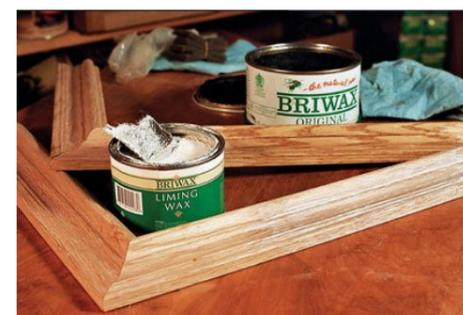
To apply liquid or paste wax, simply rub it on and wipe it off. A Scotchbrite™ pad or fine steel wool makes a good applicator; then wipe with paper shop towels. If you wipe the wax off immediately, it will leave a dull sheen as it dries. For more shine, let it dry, then buff it with a soft cloth.
