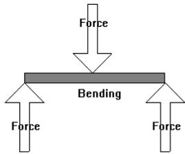
When an object bends it is under tension and compression at the same time. As seen in the diagram below, the top of the bench is experiencing compression and the bottom of the bench is under tension.
