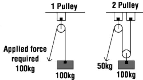
Using two or more pulleys together can change the magnitude of the force too - they can make things feel a lot lighter than they actually are. For example, one fixed pulley and one moving pulley (a block and tackle) will mean you only need half the force to pull a load. (shown above)
