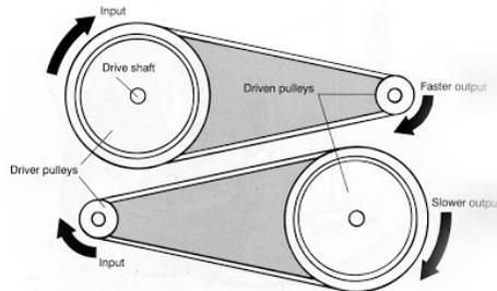
In a pillar drill, a flexible belt joins two separate pulley wheels and links the motor to the drill shaft. The belt can be put in different positions to make the drill turn faster or slower. This works in a similar way to gears - if the wheels are of different sizes, the smaller wheel will spin faster.
